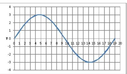
the radius of the pipe, and c is the circumference. You can use Excel to calculate the points on the curve. This plot for a 6" diameter pipe is shown in the figure. If you have a millimeter ruler it is convenient to plot y in millimeters.
