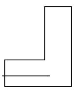
I made my rocket stove using a 2' length of 6" stove pipe. The first thing to do was to cut it on a 45° angle so the two pieces could be arranged as shown in the figure. Do this cutting before closing the pipe! The cutting line can be easily determined. Tape two pieces of printer or writing paper together and draw a straight line lengthwise in the middle. Measure the
